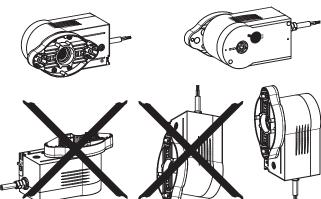
Mounting in a non-specified position can allow water ingress.
